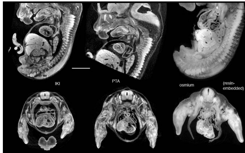
Figure 9 Mouse embryos. Left: Virtual sections of a Theiler stage 21 mouse, paraformaldehyde-fixed and IKI-stained. Voxel size 9.0 \mu\text{m} . Center: Similar embryo, PTA-stained. Voxel size 9.6 \mu\text{m} . Right: Osmium-stained 12.5 dpc mouse embryo embedded and scanned in JB4 resin (standard TEM preparation). Voxel size 8.2 \mu\text{m} . Sample was prepared by R. Walsh (Life Sciences EM Facility, Penn State University), and the microCT scan was made in 2001 at the Mayo Clinic in the laboratory of Dr. Erik Ritman (Physiological Imaging Research Lab, Rochester MN). Additional Files 4 and 5 are QuickTime movies of this PTA-stained embryo and a stage 22 IKI-stained embryo.
